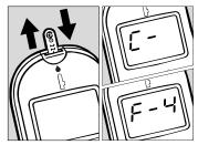
**5** Mark your Control Test result by pulling out the Test Strip, and *quickly* inserting it back into the Meter (within 2 seconds). A C- and the Function Number F# begin flashing in the Display. Marking a Control Test excludes the Control Test result from the average of stored Blood Glucose Test results.
